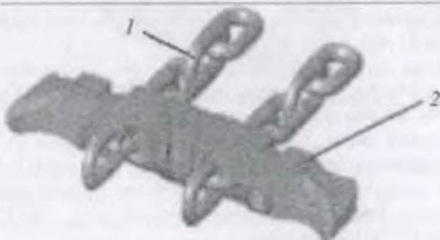
Rasm. 4.83. Kurakli konveyerining ikki zanjirli ishchi organi chiqadigan
