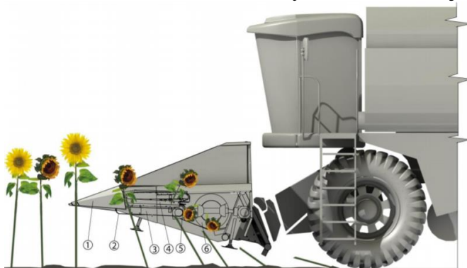
2-rasm. Moslamani umumiy ko'rinishi 1-poyani ajratgich lifter; 2-lifter; 3-urug' transporter; 4-poya transporter; 5-qirqish apparat; 6-shnek
