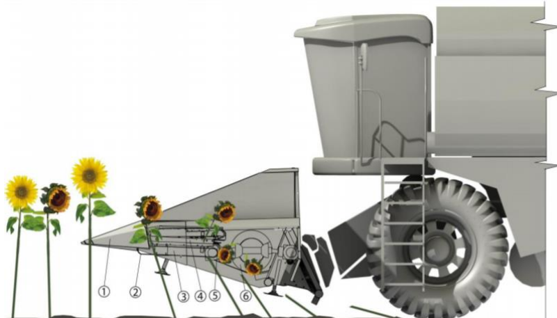
2-rasm. 1-poyani ajratgich lifter; 2-lifter; 3-urug' transporteri; 4-poya transporteri; 5-qirqish apparat; 6-shnek
