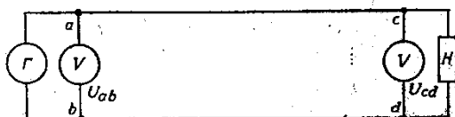
1.6- rasm. Kuchlanishni voltmترلaryordamida o'lchash
