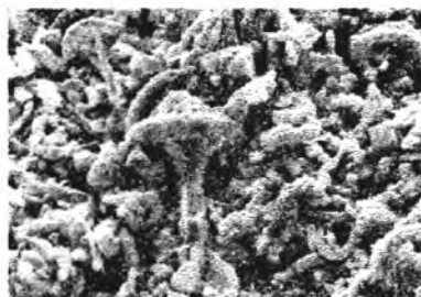
64-rasm. Yozish uchun ishlatiladigan bo'rning mikrotuzilishi (x5000).
