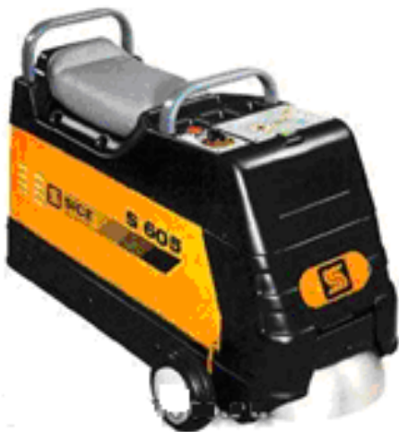
4.26-rasm. S-605 (Italiya) rusumli yengil avtomobillar g'ildiraklarini finish muvozanatlash jihozi
