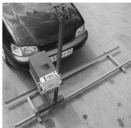
4.6-rasm. Avtomobil faralarining parametrlarini diagnostikalash uchun IPF-01 jihozi (a) va tekshirish jarayoni (b)
