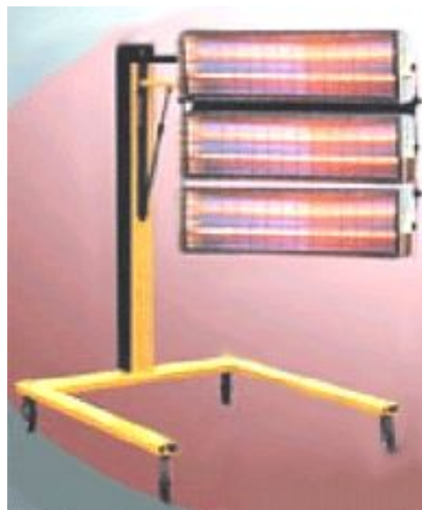
2.27-rasm. Kuzovni qisman IQ- quritish ustuni
