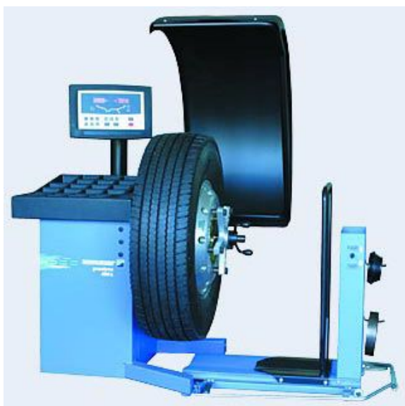
4.25-rasm Tofmann Geoduna 980L rusumidagi shinalarni muvozanatlash jihozi
