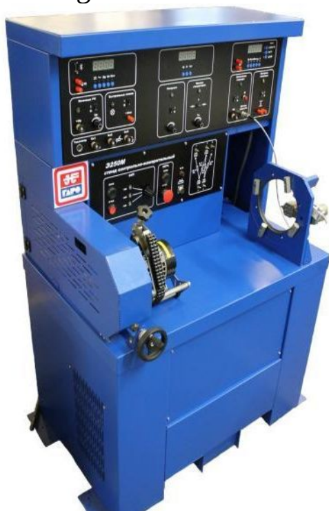
3.14-rasm. E250M-02 modelidagi generator va starterni tekshiruv-nazorat stend
