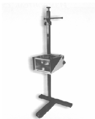
4.6-rasm. Avtomobil faralarining parametrlarini diagnostikalash uchun IPF-01 jihozi (a) va tekshirish jarayoni (b)
