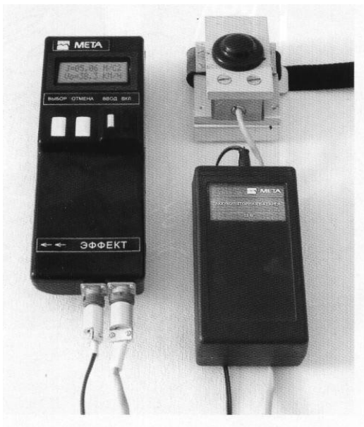
4.3-rasm. Tormoz tizimining samaradorligini aniqlovchi Effekt-02 jihozi
