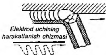
2.19-rasm. Ship choklarni payvandlash
