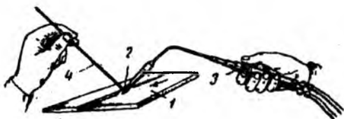
8.2-rasm. Gaz bilan dastaki payvandlash
