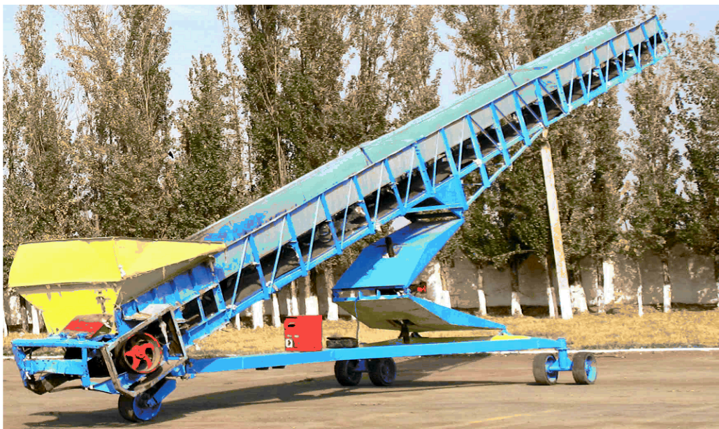
14-rasm. TTX-18. Paxtani tashuvchi lentali transporter
