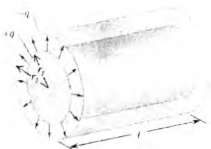
18.5-rasm. Silindrik kondensatorning tuzilishi
