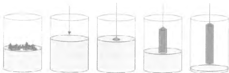
3.9-rasm. Si monokristallini Choxralskiy usuli bilan o'stirish qurilmasining tasviri: 1 – Si zatrovkasi, 2 – Si monokristalli, 3 – \text{SiO}_2 qozoni, 4 – Si eritmasi, 5 – grafitli ushlagich, 6 – qizdirgich, 7 – inert gaz (Ar)
