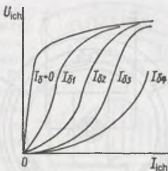
7.24-rasm. Turli qiymatdagi boshqarish toklari I_b ga tegishli U_{ich} = f(I_{ich}) egri chiziqlari, U_{ich} — ish chulg'amida I_{ich} tokidan kuchlanish tushuvi.
