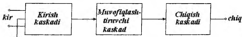
9.15-rasm. Uch kaskadli OK funksional sxemasi.
