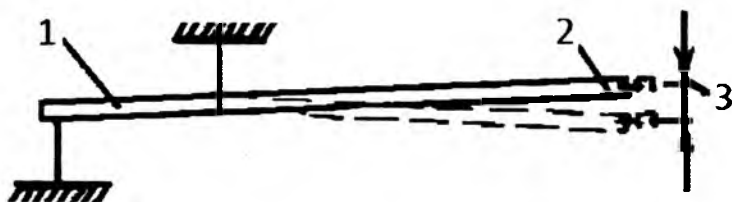
62-rasm. Shtanganing egiluvchanligini sinash tartibi:
