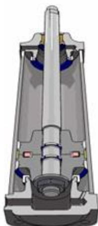
3.2.12-rasm. 3D-formatdagi pnevmatik porshenli silindr qirqimi
