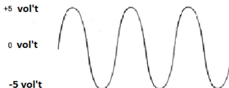
Rasm 5.2 +5, -5 amplitudali o'zgaruvchan tokning sinusoidal signali
