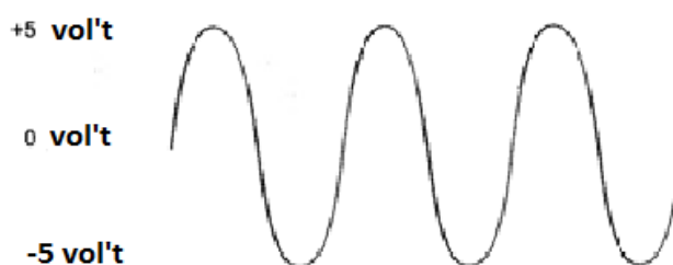
Rasm 13.2 +5, -5 amplitudali o'zgaruvchan tokning sinusoidal signali
