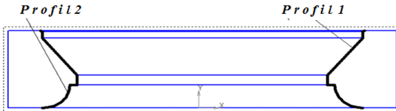
3.24-rasm. Shakldor keskich kesuvchi qirrasi profilini qurish
