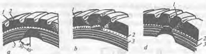
3.52-rasm. Shikastlangan joyni kesish shakllari: a —ichki konussimon; b —tashqi konussimon; d —qarama-qarshi konussimon; 1—protektor; 2—breker; 3—karkas.
