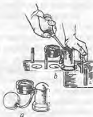
3.14-rasm. Klapan va uning egarini tozalash sifatini tekshirish:
