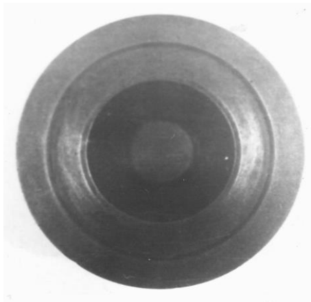
7.13-rasm. Matritsa ishchi qismi qattiq qotishma BK6
