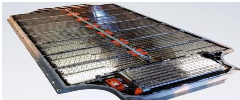
4-rasm. Elektromobilda qo'llaniladigan litiy-ionli akkumulyator
