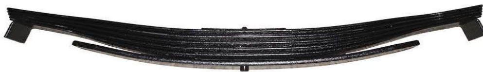
2-rasm Ko'priikka qo'shimcha ressor qo'yish
