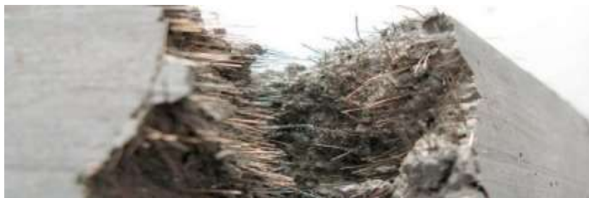
Rasm 5. Tolalar bilan mustahkamlangan toshning sinishi
