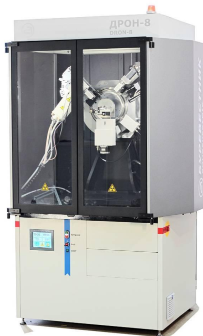
B- DRON-8 rentgen diffraktometri, vertikal \Theta - \Theta goniometrli, Sankt-Peterburg (2010 y.)
