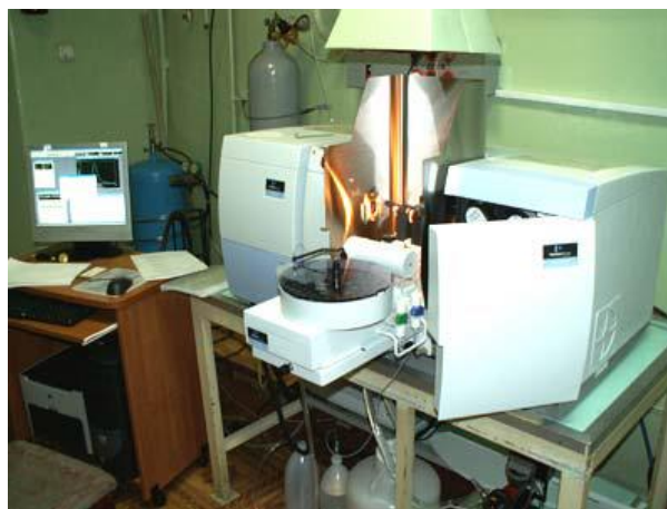
106-rasm. Elektrotermik atomizator bilan ishlash. AAnalyst-400 spektrometri (Perkin-Elmer, AQSh).
