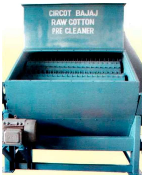
36-rasm. Qiya tozalagichning ochiq ko‘rinishi (Tuhfa:. M / s Bajaj Steel Industries Ltd.)
