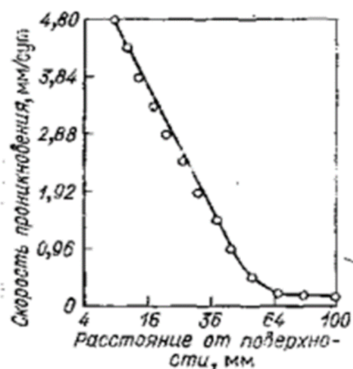
Rasm 5.7. H_2SO_4 eritmasining granit-porfir jinsiga chiqur kirib borish tezligining o'zgarishi
