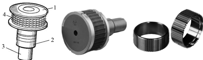
202-rasm. Diskretlovchi barabancha: 1 – barabancha; 2 – podshipnik; 3 – blokcha; 4 – arra tishli garnitura
