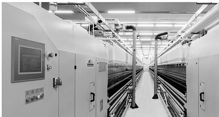
191-rasm. Halqali yigirish mashinasida momiq va changni tozalash qurilmasi
