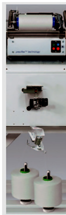
5.24-rasm. SSM TW2-D DIGICONE® preciflex™ turidagi qo‘shib o‘rash mashinasi
