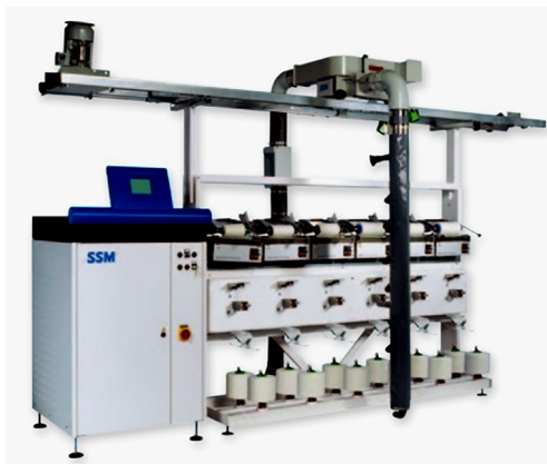
5.24-rasm. SSM TW2-D DIGICONE® preciflex™ turidagi qo‘shib o‘rash mashinasi
