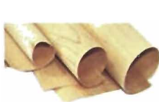
6.14-rasm. Yog'ochni qatlamlarga ajratib shilish (a) va ularni o'zaro yopishtirib (b) faner tayyorlash:
