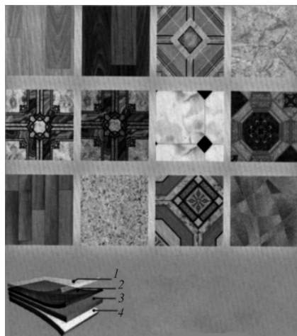
10.7-rasm Har xil ranglagi manzarali O'zbekiston linoleumlari: 1. Ustki qoplama, 2. Rasmlı qatlam, 3. PVX qatlami, 4. Yumshoq asos-EKOPOL.
