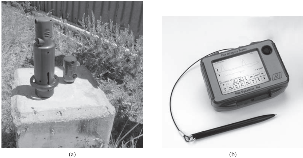
Figure 23.10 Low strain sonic echo equipment being used on a 300 mm (12 in) concrete driven pile: (a) a small drop hammer (left) and wireless accelerometer (right rear) and (b) hand-held data processing unit. (b courtesy of Pile Dynamics, Inc.)
