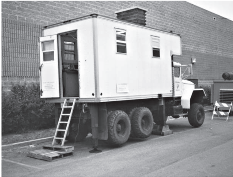
Figure 4.21 A truck-mounted CPT rig. A hydraulic ram, located inside the truck, pushes the cone into the ground using the weight of the truck as a reaction.
