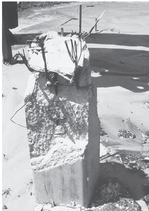
Figure 19.4 These piles were damaged during driving because the contractor selected a hammer that was too large. A driveability analysis could have predicted these problems, and would have helped the contractor select a more appropriate hammer (courtesy of GRL Engineers, Inc.).
