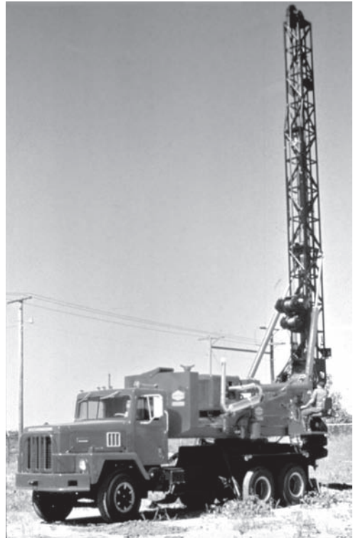
Figure 12.29 Typical drilling rig for constructing drilled shafts. This rig is able to drill shafts up to 1,800 mm (72 in) in diameter and 24 m (80 ft) deep (ADSC: The International Association of Foundation Drilling).
