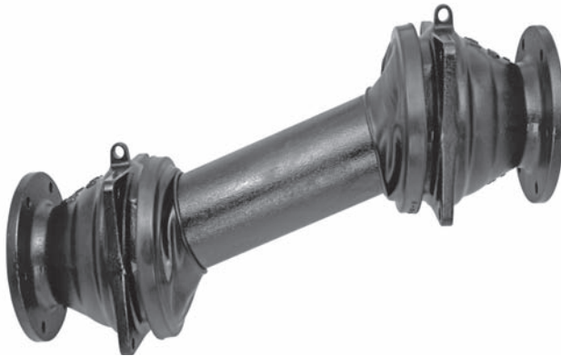
Figure 5.6 This flexible, extendible pipe coupler has ball joints at each end and can telescope to allow lengthening or shortening. These couplers can be installed where utility lines enter structures, thus accommodating differential settlement, lateral movement, extension, and compression. For example, a 203 mm (8 in) diameter connector can accommodate differential settlements of up to 510 mm (20 in) (Courtesy of Romac Industries, Inc.).
