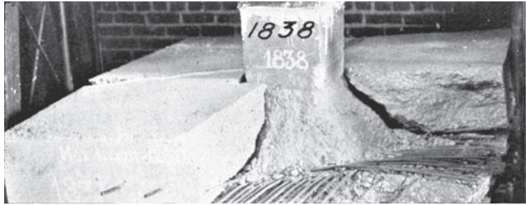
Figure 10.2 “Shear” failure in a spread footing loaded in a laboratory (Talbot, 1913). Observe how this failure actually is a combination of tension and shear. Source: Board of Trustees of the University of Illinois.
