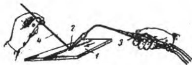
2.1.2-rasm. Gaz bilan dastakli payvandlash.
