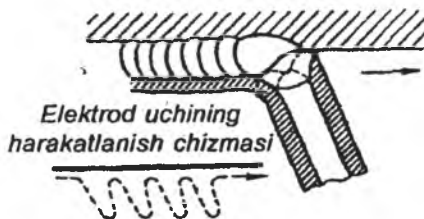
1.2.28-rasm. Ship choklarni payvandlash.
