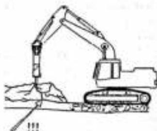
15-rasm. Toshni (a) portlatish usulida va (b) maksus mashinalarda qazib olish
