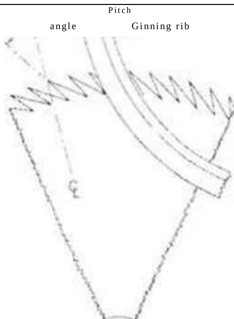
Fig. 6.3 Schematic diagram showing the orientation of rib with respect to saw discs.
