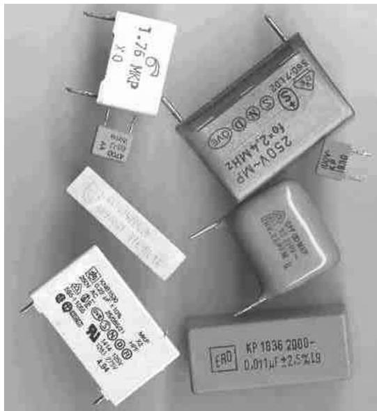
**Figure 4.3.** A selection of polypropylene capacitors
