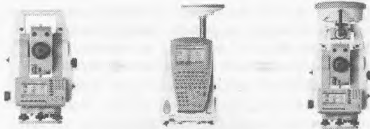
2.12-rasm. Smart Station sistemasi
