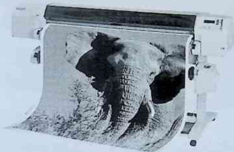
6.5.25-rasm. Katta bichimli ko'p rangli purkovchi bosma tizimi; imkonlilik qobiliyati 600 dpi, bosma kengligi 1340 mm (DesignJet 3000 CP, HP)
