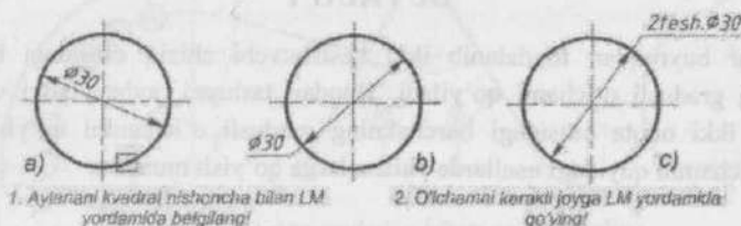
8.17-rasm. Aylanaga diametrli o'lcham qo'yish.
