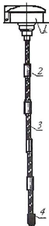
17-rasm. Termoosilma: 1 – boshcha; 2 – oraliq termometr; 3 – egi-luvchan tross; 4 – oxirgi termometr.
