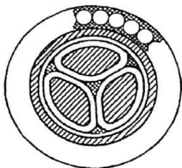
27-rasm. Bronya qatlami bilan himoyalangan yuqori kuchlanishli kabel.
