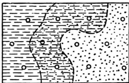
5.26-rasm. Turli tog' jinslari ajratilgan uchastkalarni xaritada ifodalanishi (A.M.Agadjanov, 1958): 1 – qumtosh; 2 – alevrolit; 3 – argillit
