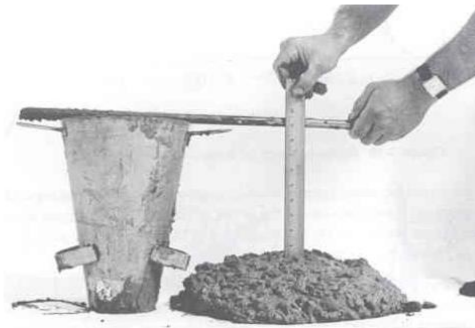
8.13-rasm. Tuproqning tarqalishini aniqlash
