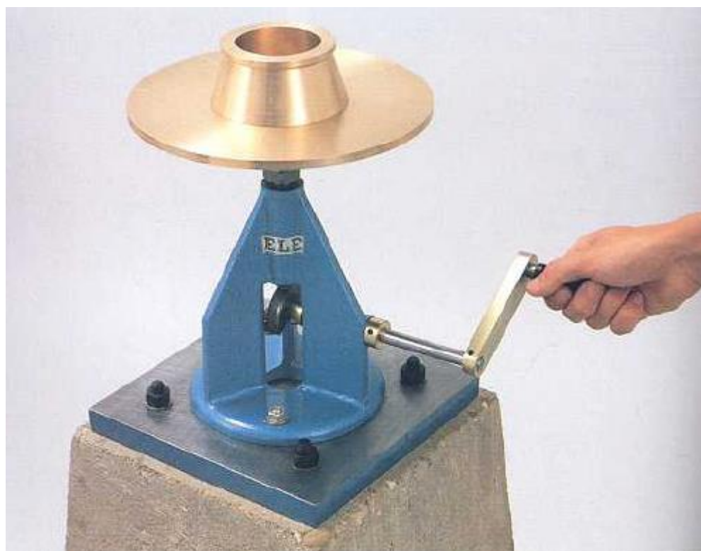
8.6- rasm . Chayqaladigan stol va konusning holati
