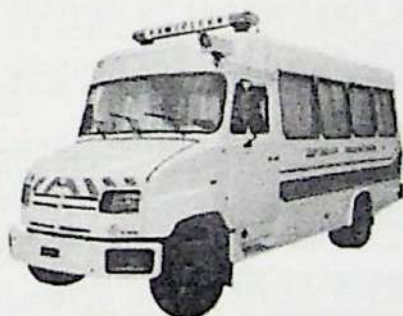
7.7-rasm. Videoyozuv tizimli avtomobilida KP-514MP mobil laboratoriyasi
