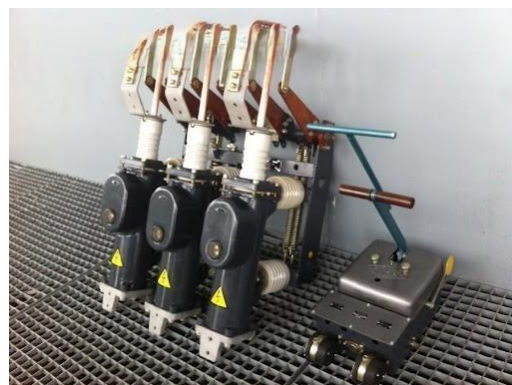
6.31-rasm. PRBA-114 yuritmasi VPM-10 markali, kam moyli uzgichda qo'llanilishi.
