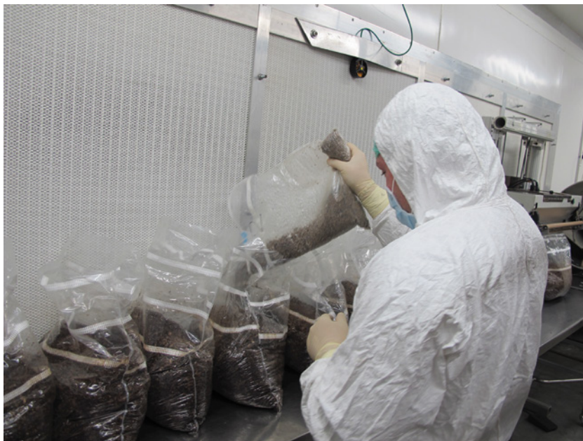
Figure 5.5 Manual inoculation of large grain spawn bags in front of laminar flow. Note the anemometer measuring the horizontal LAF's air velocity at the top and the sealing machine at the right.
