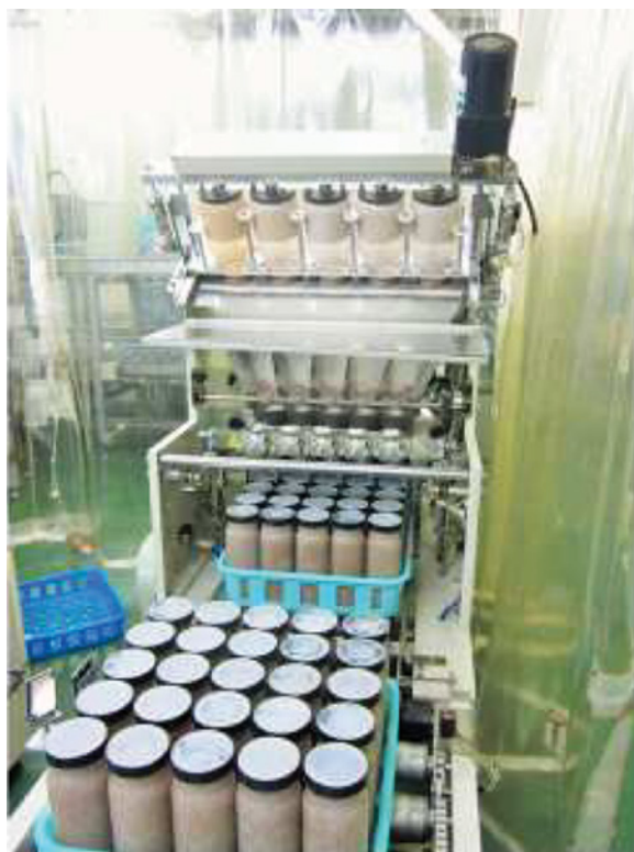
Figure 15.9 Automatic inoculation machine for bottle cultivation.
