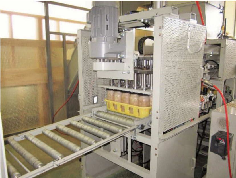
Figure 15.6 Automatic filling machine for bottle cultivation.
