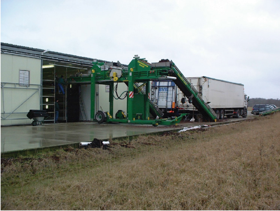
Figure 9.9 An actual situation in the Netherlands where they fill phase III compost plus supplement and casing using modern equipment all together on a typical modern Dutch mushroom farm. In roughly 1 hour they fill about 200–300 m 2 with these materials. The organization is so good that the head filling machine (from a special filling company) plus the truck with compost and the truck with casing soil, from different companies, arrive at the same time. Just 90 minutes later, everything is gone and the room is filled perfectly.
