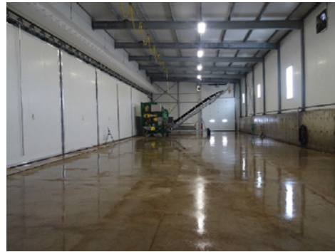
Figure 6.14 Left: Filling cassette for phase II tunnels. Right: Pulling winch for emptying compost from open tunnel floors with nylon nets.
