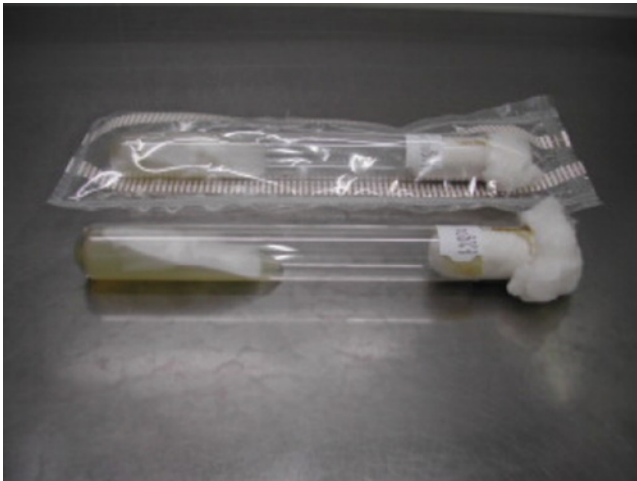
Figure 5.11 Double-packing cultures in fridges limits risks of cross-contamination.
