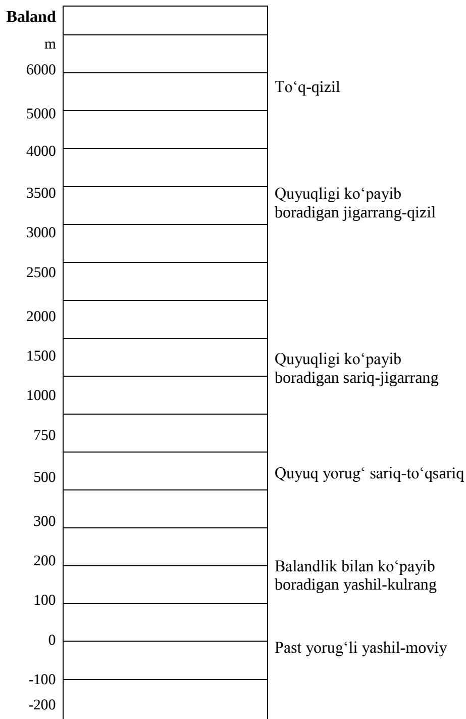
66-rasm. Gipsometrik shkalani qurish sxemasi
