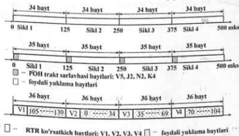
6.7-rasm. C-12 (a), VC-12(6) va TU-12 (v) yuqori sikllarga birlashish
