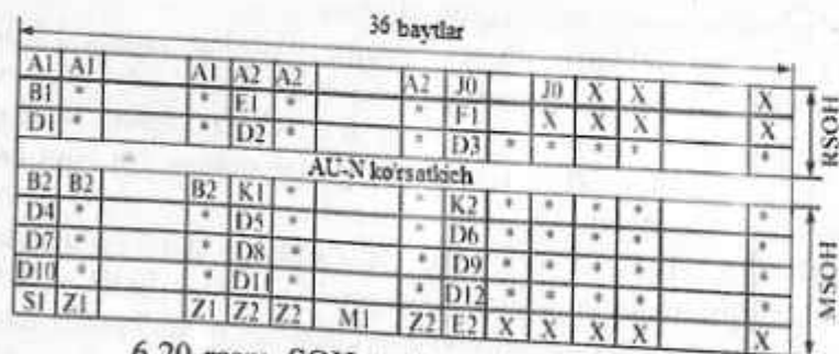
6.20-rasm SOH strukturasi STM-4 sikli uchun
