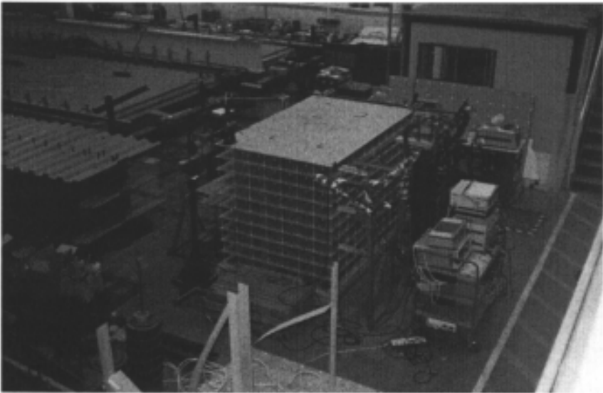
Fig. 10.9 Dynamic tests: model 'M2' and the vibrator.
