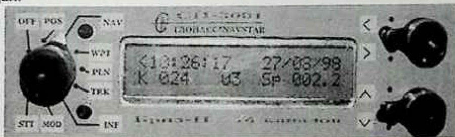
6.12-rasm. CH-3001 qabullash indikatorining old ko'rinishi
