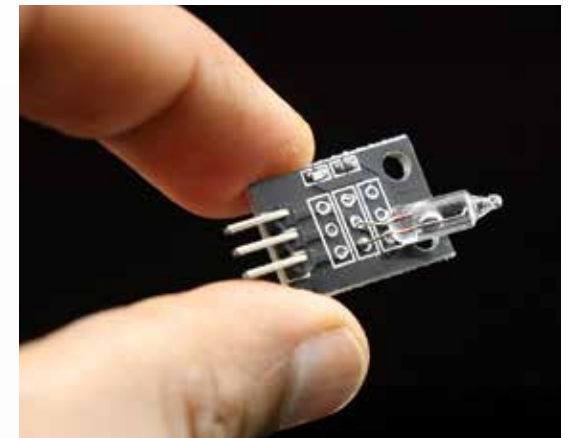
Tilt switch sensor modules are commonly used in lifting, mining, and construction equipment to detect potential instability, tipping, or rollover and alert machine operators.
