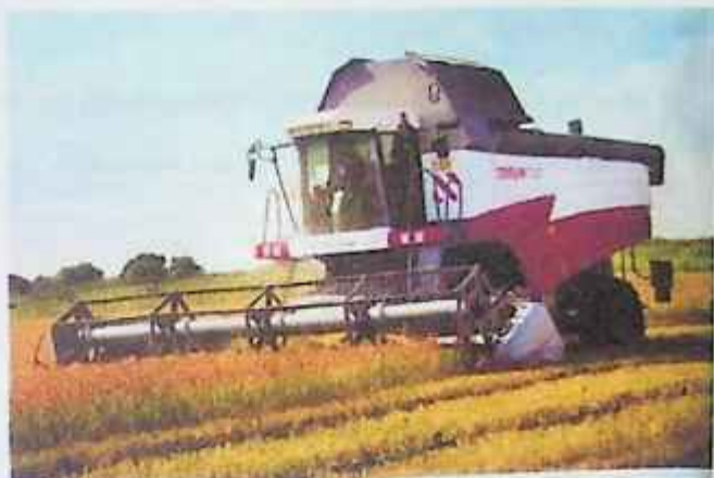
25-rasm. TORUM-740 rusumidagi g'alla-don ekinlarini yig'ish kombayini
