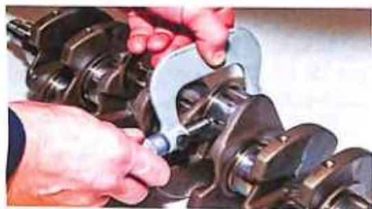
14-rasm. Mikrometr MK 50-1 bilan detalni o'lchash.
