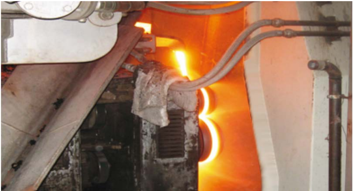
4.9-rasm – ISOROC ishlab chiqarishda tola hosil bo‘lishi
